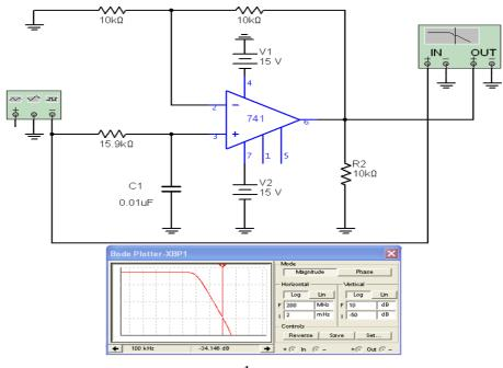
The cut-off frequency is given by  $f_c = \frac{1}{2\pi RC}$ . Here, R = 15.9K and C= 0.01uF.
