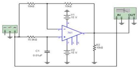
This is nothing but like a first order low pass filter (*Which you have seen in question no. C*), the only difference is that the grounded 10K resistor is connected to the input.
