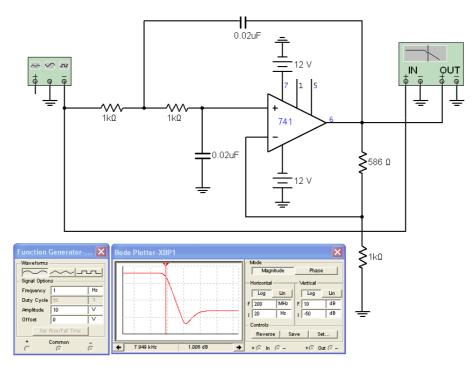
The feedback capacitor ( $C_A$ ) provides the feedback for shaping the response near the edge of the pass band.
