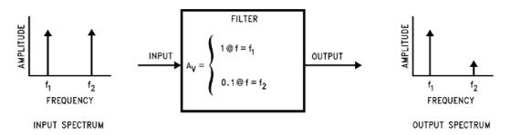
The voltage transfer function of a filter is defined by  $H(S) = V_{OUT}(S) / V_{IN}(S)$ . The transfer function for n<sup>th</sup> order network (one with 'n' capacitors and inductors) is defined by
