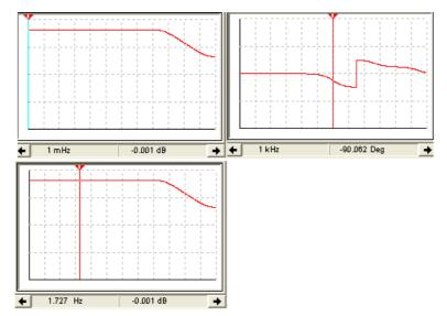
Note the upper frequency limitation by op-amp and note the gain of the filter.
